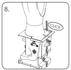
Test the bollard is secure by attempting to lift from the socket.
